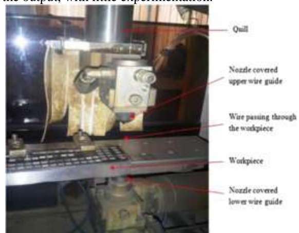
Figure 4 - Experimental setup of the WEDM
